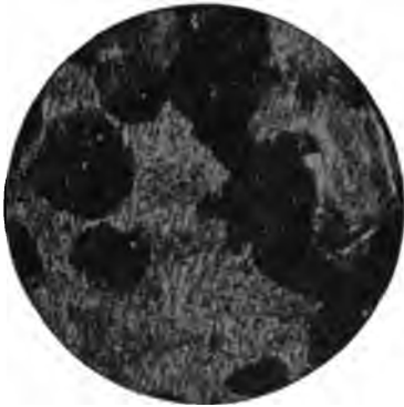
Fig. 27. Quenching Oil too Hot; Troostite and Martensite Structure
